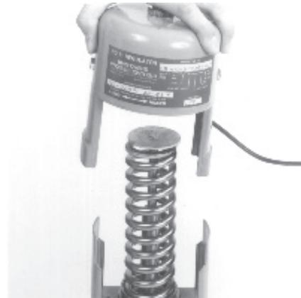
7. Remove Housing and Thermal System
