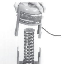
7. Remove Housing and Thermal System
