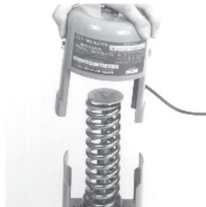
7. Remove Housing and Thermal System
