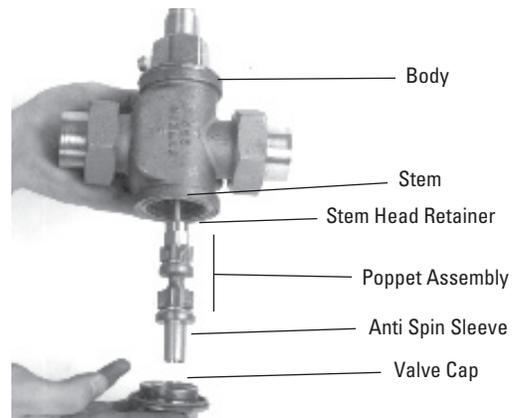
12A. (RA, 1" to 2" ) remove valve cap
