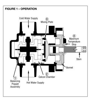
NOTE: Following any maintenance of unit, maximum temperature stop must be reset. See page 5 for instructions.
