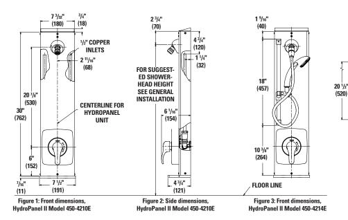
Installation should be in accordance with acceptable plumbing practices. Flush all piping thoroughly before installation. Failure to do so can result in valve malfunction. Before installation of HydroPanel<sup>™</sup> II, rotate the stem or handle off.
