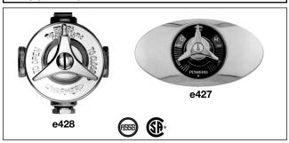
The Series e427 and e428 HydroGuard valves automatically mix hot and cold water to deliver blended water at any desired temperature within a specified range. The assembly contains an advanced thermal actuators which maintains the selected water temperature within rigid tolerances despite temperature and pressure fluctuations in the water supply.
