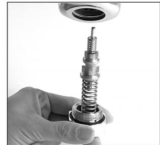
Remove body cap with wrench to service cold water assembly. **NOTE: Cap is spring loaded. Remove with caution.**
