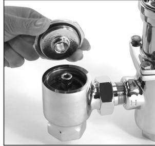
Remove bonnet with 2-1/4" (57mm) wrench or use a 3/4" socket wrench.
