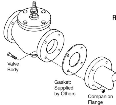
Figure 6 - Installation of Flanged End Valves
