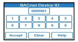
To change the BAC-MSTP Address, press the words **BAC-MSTP Address**, enter the address, and press **ACCEPT**.
