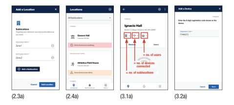
Starting at the controller, register device and connect to network. A Registration Code from the device is required to set up the app.
