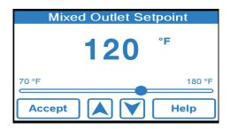
Selecting and Setting Outlet Water Temperature Set-point:
