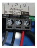
5. Remove the Actuator Cables from the control box.
