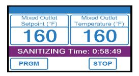
9. After Sanitization Mode has completed (user selected run time has elapsed), the IntelliStation will go into a Cool Down Mode to return to the Mixed Outlet temperature prior to returning to normal operation.
