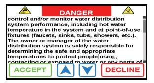
3. You must touch the ACCEPT icon to proceed to the Programming Menu and to use system functions. Touching the DECLINE icon means you will not be able to change system settings and you accept all default settings (including the outlet water temperature set point of 140° F/ 60° C) as safe and appropriate for the water distribution system users and the facility. You will be returned to the "Programming" screen.
