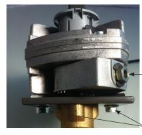
**Armature Clamping Nut**
