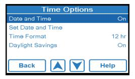
To select time format, toggle to the 12hr or 24hr radio button and select ACCEPT
