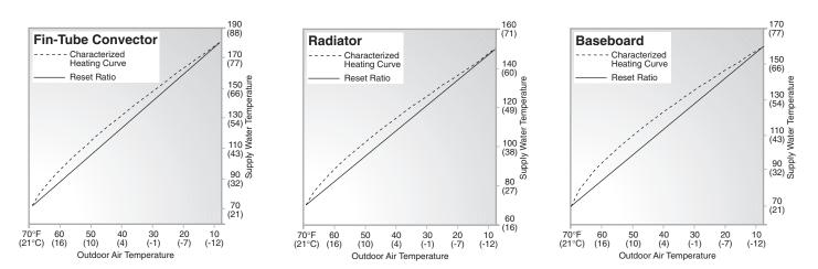
Not all heating terminal units behave in the same manner. Because of this fact, applying a generic outdoor reset strategy, such as a Reset Ratio, cannot provide the maximum performance and comfort from the heating system. A reset strategy that is customized to the heating system, such as a Characterized Heating Curve, will provide better performance and comfort.
