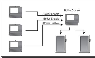
When multiple controls in a single system try to operate the boiler(s) simultaneously, short cycling can occur. For the most efficient boiler operation, only one control should operate the boiler(s). All of the remain-
