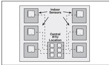
Remote sensing allows the end user to control the indoor temperature of several zones from one central location. Multiple indoor sensors located throughout the building measure the zone temperatures. Each sensor is
