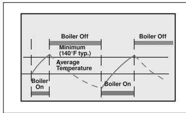
During mild outdoor temperatures, low supply water temperatures are desired in order to prevent overheating in the building. Most boilers must be operated at temperatures above the flue gas dew point to prevent condensation.
