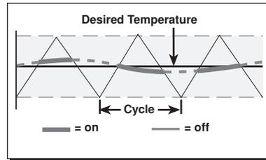
Pulse Width Modulation (PWM) is an on / off action that differs from an on / off differential by changing the length of the "on" time based on how much the actual temperature differs from the desired. The heating device is operated
