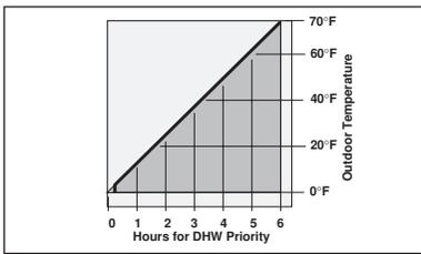
If DHW priority is selected then heat to the heating system is stopped during a call for DHW. At cold outdoor temperatures the building may freeze up when there is a long call for DHW. In order to prevent this, the control must
