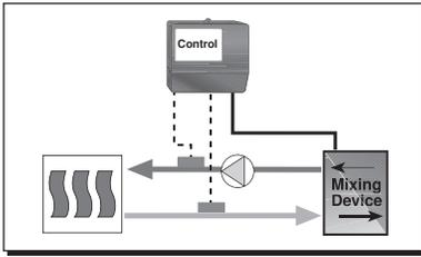
Snow melting systems deal with extreme temperature differences. Slab protection is provided by limiting the rate of heat transfer into the slab. This is done by slowly ramping up the temperature difference ( $\Delta T$ ) across the slab
