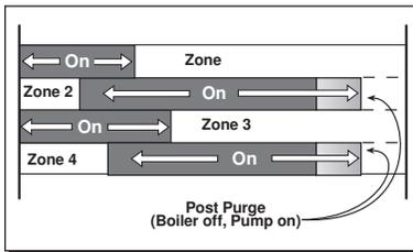
Since a Zone Control calculates all the on times of the zones, a Zone Post Purge can be performed. Before the last zone is turned off in a heating cycle, the boiler is turned off but the zone continues to draw heat from the
