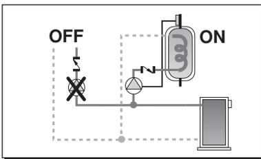
DHW priority allows the DHW tank to recover faster by temporarily suspending the heat supply to the heating system. All of the available heat is provided to the DHW tank for a period of time. This function provides more
