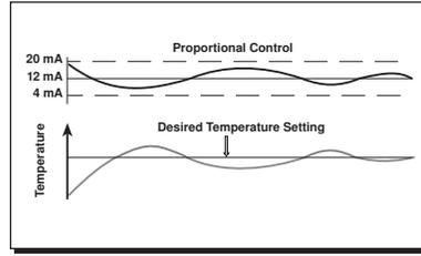
A modulating output provides a signal which is directly proportional to the actuator position required by the control. Common modulating output signals are a 4-20 mA, 0-135 Ω, or 2-10 V(dc). These signals can also be used to
