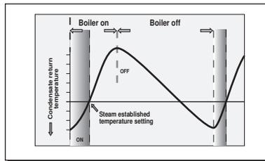
In steam systems the boiler is operated in heating cycles which are dependent on the outdoor temperature. Each heating cycle starts when the system is filled with steam. The Steam Established function delays the
