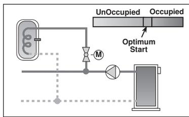
To ensure that the DHW tank is up to temperature after the DHW Setback period the control must raise the tank temperature before the setback period ends. This can be accomplished automatically by using a control
