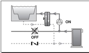
Setpoint Priority allows the setpoint load to recover faster by temporarily suspending the heat supply to the heating system. All of the available heat is provided to the setpoint load for a period of time. This function
