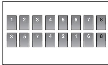
When multiple boilers are staged and rotated, the last stage can be fixed to fire last. A common application is to allow a second boiler plant, such as a DHW boiler plant, to assist with the heating when the DHW system is
