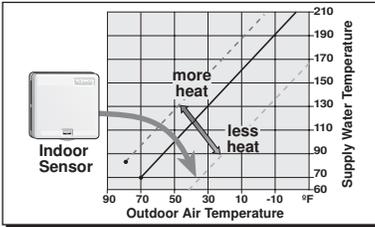
Most buildings have internal heat gains and losses due to people, passive solar heating, or opening of doors. If only the outdoor temperature is measured, the control cannot compensate for these heat gains/losses
