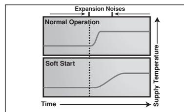
When a sudden change of supply water temperature occurs, the heating system is subjected to thermal stresses. This is evident in expansion and contraction noises. A change in supply water temperature results from
