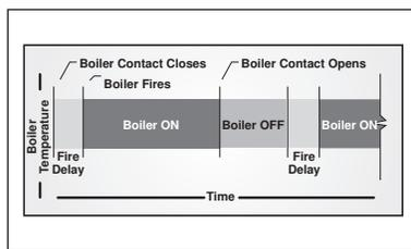
Most boilers have built in safety delays before the burner is allowed to fire. The Fire Delay function allows a boiler staging control to account for the delay between the time that the control signals the boiler to operate and
