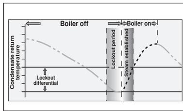
In order to increase the efficiency of a steam system, a Lockout or cool down period before each heating cycle can be used. The lockout differential ensures that the condensate temperature drops before turning the
