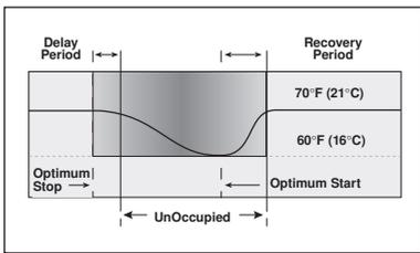
When a setback schedule is in effect, the building experiences delays in dropping down its temperature at the beginning of the setback period, and increasing its temperature at the end of the setback period. The Optimum
