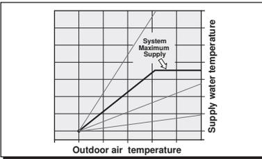
Some systems such as radiant floor heating must be maintained below an allowable maximum temperature in order to protect the tubing or flooring surface. System protection can be achieved by limiting the supply water
