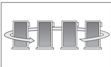
This function rotates the firing sequence of a group of staged boilers based on the accumulated running hours of each stage. When one stage has accumulated 48 hours more running time than any other stage, the oper-
