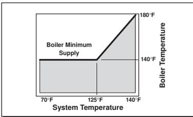
Many systems, such as radiant heating, use a mixing device to reduce the system supply water temperature. The boiler in these systems should be operated at the minimum allowable water temperature in order to reduce
