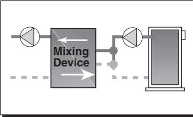
To protect the boiler against flue gas condensation and thermal shock, a mixing device should be used to control the load on the boiler. If the temperature of the boiler is below the condensation temperature or the return
