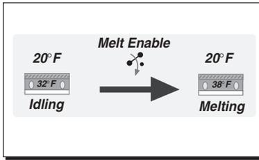
In systems where snow and ice removal is critical, such as hospital ramps, the pick up time for a snow melting slab can be reduced by maintaining the slab at an idling temperature. The idling temperature may be just
