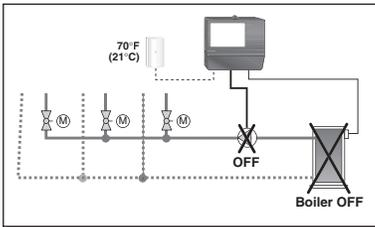
When the outdoor air temperature is warmer than the indoor temperature, no additional heat is required in the building and therefore the heating system can be shut down. Warm Weather Shut Down (WWSD) provides
