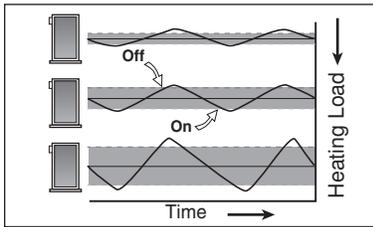
In order to decrease temperature swings and increase boiler efficiency, this function automatically changes the on / off differential of the boiler based on the heating load. As the load increases, the differential will decrease to
