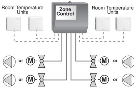
In general, there are two types of control systems that are used to operate zones in a heating system. These two types are individual thermostats or an integrated zone control with room temperature units (RTUs).
