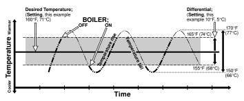
Fig. 6 Bang-Bang (On/Off) function
