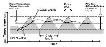
Fig. 7 Pulse Width Modulation function
