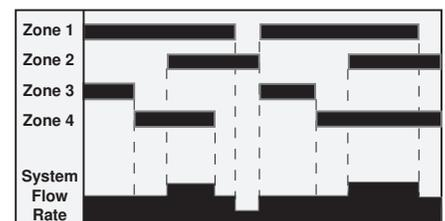
Figure 4. Integrated Water Flow Control (Central Zone Control)
