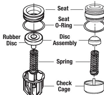
Note: Rubber seat disc can be replaced. However, disc holder and disc retainer are permanently bonded to prevent failure.
