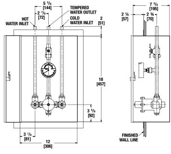
Note: Dimensions are shown  $\pm \frac{1}{2}$ " Dimensions in parentheses are in mm
