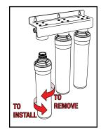
completely once to remove any natural carbon fines from the UF Drinking system. Check over the next 24 hours to ensure no leaks are present.
