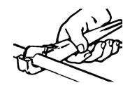
Cut the tube square. It is essential that the outside diameter be free of score marks and that burrs and sharp edges be removed before inserting into fitting.
