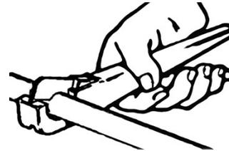
Cut the tube square. It is essential that the outside diameter be free of score marks and that burrs and sharp edges be removed before inserting into fitting.
