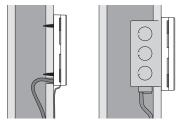
The enclosure is either mounted flush onto a wall or it can be placed onto a 2" x 4" non-conductive electrical box. The mounting holes in the enclosure accept #6 screws. Wiring to the control enters the wiring chamber through the back or bottom of the enclosure.
