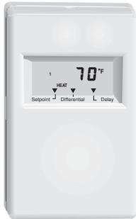
The tekmar Two Stage Setpoint Control 152 is a microprocessor-based control that can be programmed with two independent setpoint temperatures to cycle heating or cooling devices on and off.
