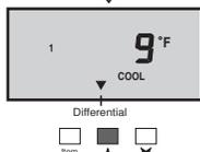
Push and Hold the V button. The programmed Delay 1 and then Delay 2 will be displayed.
