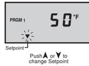
Pushing the "Item" button changes the flashing pointer to Differential (1)
