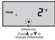
Pushing the "Item" button changes the flashing pointer to Delay (2)
