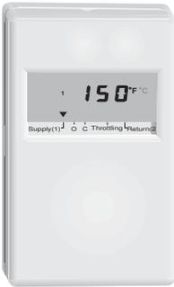
The tekmar Mixing Setpoint Control 153 is a microprocessor-based control with a floating action output intended to operate a mixing valve, damper, etc. through an actuating motor.
