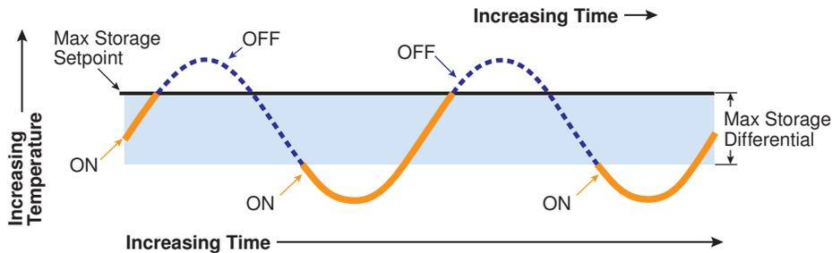
Relay operation showing the turn on and turn off points with respect to the Max Storage Setpoint and Differential.
