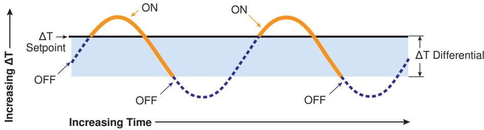
Relay operation showing the turn on and turn off points with respect to the  $\Delta T$  Setpoint and  $\Delta T$  Differential.
