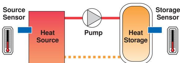
The Difference Setpoint Control 156 has two control points; heat source and storage. The heat source could be a solar collector or wood boiler while the heat storage is typically a storage tank. The control is looking at the temperature difference ( $\Delta T$ ) between the source and storage to determine when to close the relay and start the heat transfer. The setpoint operation that follows will explain the on and off points of the relay.
