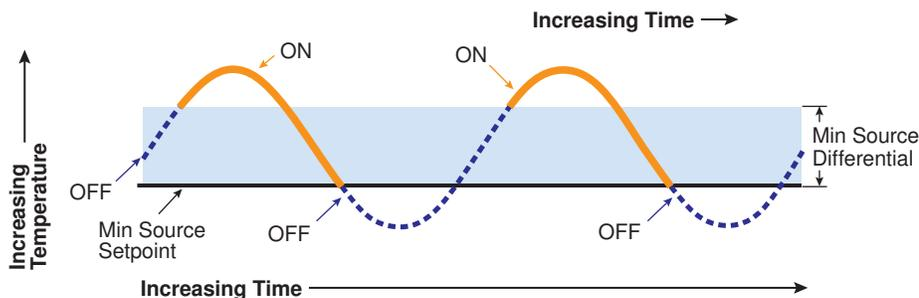
Relay operation showing the turn on and turn off points with respect to the Min Source Setpoint and Differential.
