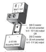
Converting the 0 - 20 mA Output to Operate a 0 - 10 V (dc) Device
