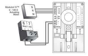
The 4 to 20 mA output can be converted to a 0 - 135  $\Omega$  output for a V9055<sup>TM</sup> gas valve actuating motor using a 0 - 135  $\Omega$  tekmar Converter 005 (sold separately).
