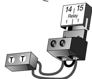
If a boiler pump is connected to the *Relay 1* terminals (14 and 15), make sure that power to the terminal block is off and install a jumper between the terminals. When power is applied to circuit, the boiler pump should start. If the pump does not turn on, check the wiring between the terminal block and pump and refer to any installation or troubleshooting information supplied with the pump. If the pump operates properly, disconnect the power and remove the jumper.
