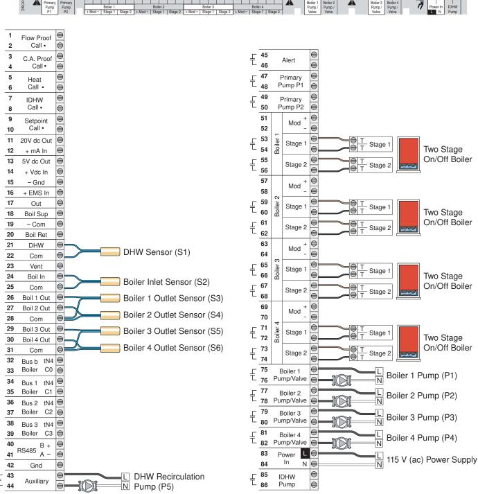
Two modulating condensing boilers are operated to provide heat for a space heating load. The boiler target temperature for the space heating load is determined from outdoor temperature reset and indoor temperature feedback provided by tekmarNet® thermostats. One of the boilers (boiler #4 output) also operates to provide heat for an indirect DHW load with priority over space heating.
