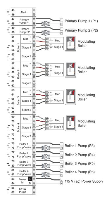
Four two-stage non-condensing boilers are operated to provide a fixed setpoint temperature for a dedicated DHW load. The DHW recirculation pump can optionally be operated on a schedule to save energy.
