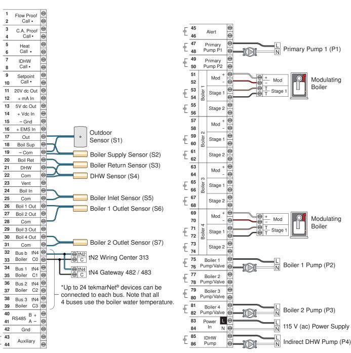
Two modulating non-condensing boilers are operated to provide a boiler target temperature for space heating and indirect DHW loads. The boiler target temperature for the space heating load is determined from outdoor temperature reset and indoor temperature.
