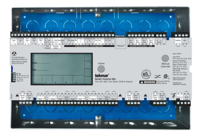
Two single stage non-condensing boilers & two modulating condensing boilers are operated to provide a boiler target temperature for space heating, indirect DHW and setpoint loads. The boiler target temperature for the space heating load is determined from outdoor temperature reset.
