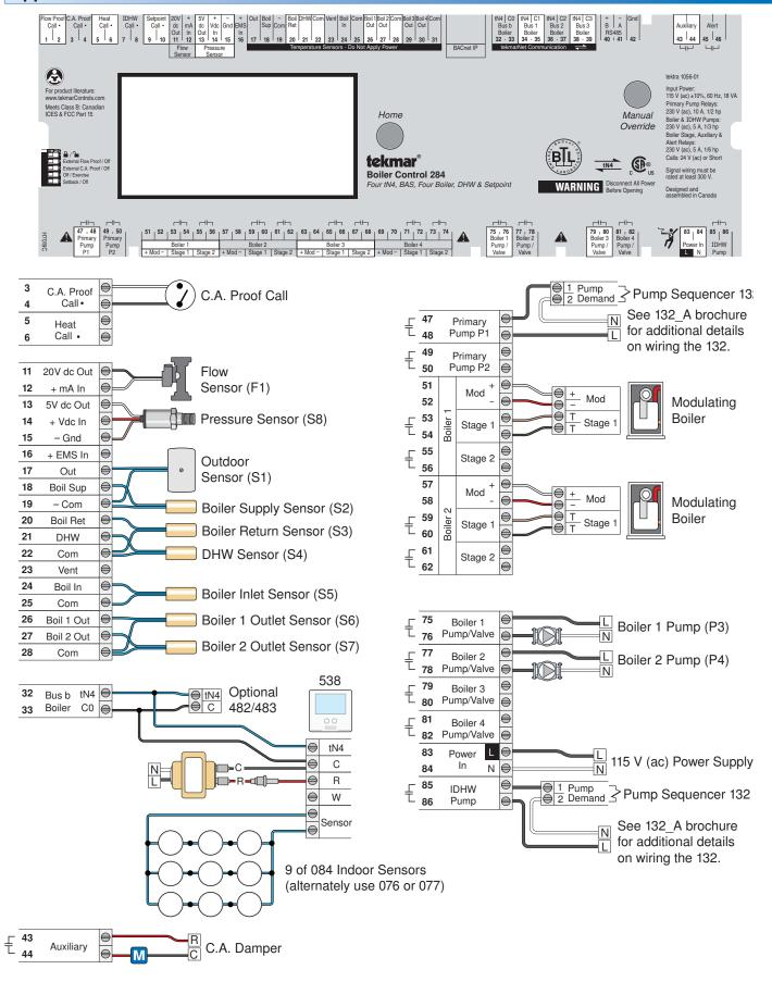
Four modulating condensing boilers are operated to provide an outdoor temperature reset boiler target for a space heating load.
