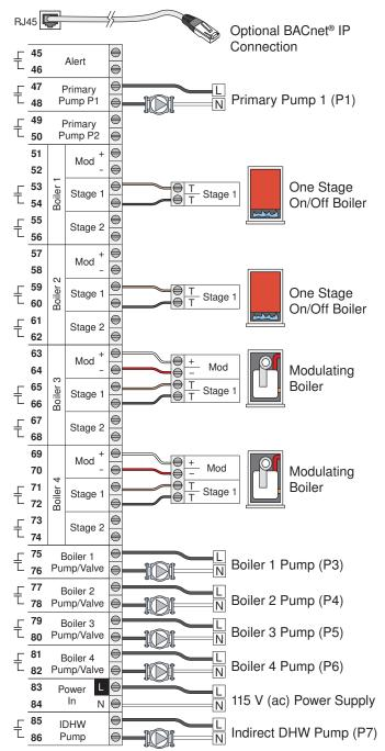
Four modulating condensing boilers are operated to provide an outdoor temperature reset boiler target for a space heating load.
