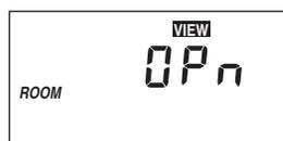
The control is no longer able to read the indoor sensor due to an open circuit. The control will continue to operate as if there was nothing connected to the indoor sensor input. Locate and repair the problem as described in the Data Brochure D 074. If the indoor sensor is deliberately removed, the control must be powered down, and then powered back up. To clear the error message from the control after the sensor has been repaired, press the **Item** button.
