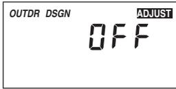
Press and release the **Item** button to advance to the OUTDR DSGN adjustment. Press and hold the **▲** button until OFF is displayed.
