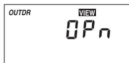
The control is no longer able to read the outdoor sensor due to an open circuit. In this case the control assumes an outdoor temperature of 32°F (0°C) and continues operation. Locate and repair the problem as described in the Data Brochure D 070. To clear the error message from the control after the sensor has been repaired, press the **Item** button.
