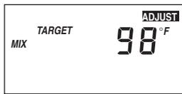
Press and release the **Item** button to advance to the MIX TARGET adjustment. Use the **▲** or **▼** button to select the desired temperature. The MIX TARGET setting is set to the desired setpoint supply temperature.
