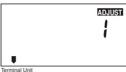
Press and release the **Item** button to advance to the *Terminal Unit* adjustment. Use the ▲ or ▼ button to select the desired terminal unit. The terminal unit number corresponds to the type of terminal that is being used. The table below lists the terminal units and their default values.
