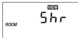
The control is no longer able to read the indoor sensor due to a short circuit. The control will continue to operate as if there was nothing connected to the indoor sensor input. Locate and repair the problem as described in the Data Brochure D 074. To clear the error message from the control after the sensor has been repaired, press the **Item** button.
