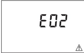
The control has an internal sensor that monitors the temperature inside the enclosure. The internal sensor has a short circuit that is not field repairable. Contact your tekmar sales representative for details on the repair procedures if this error occurs.
