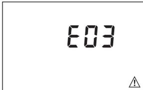
The control has an internal sensor that monitors the temperature inside the enclosure. The internal sensor has an open circuit that is not field repairable. Contact your tekmar sales representative for details on the repair procedures if this error occurs.
