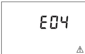
The control has an internal sensor that monitors the temperature inside the enclosure. The internal temperature of the control is too hot. The control will shut off both variable speed outputs until the control has cooled off. Make sure the ambient temperature is less than 120°F (50°C). To clear the error message from the control after the control has cooled off, press any button.
