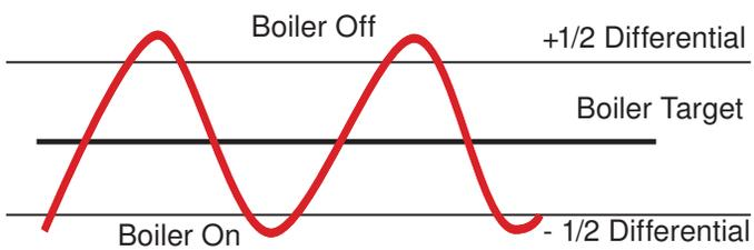
In order to decrease temperature swings and increase boiler efficiency, the Auto Differential feature automatically adjusts the operating differential of the boiler based on the heating load. As the load increases, the differential will decrease to minimize temperature swings. As the load decreases, the differential will increase to prevent short cycling. This can significantly improve operating efficiency and prevent equipment failures through excessive cycling.
