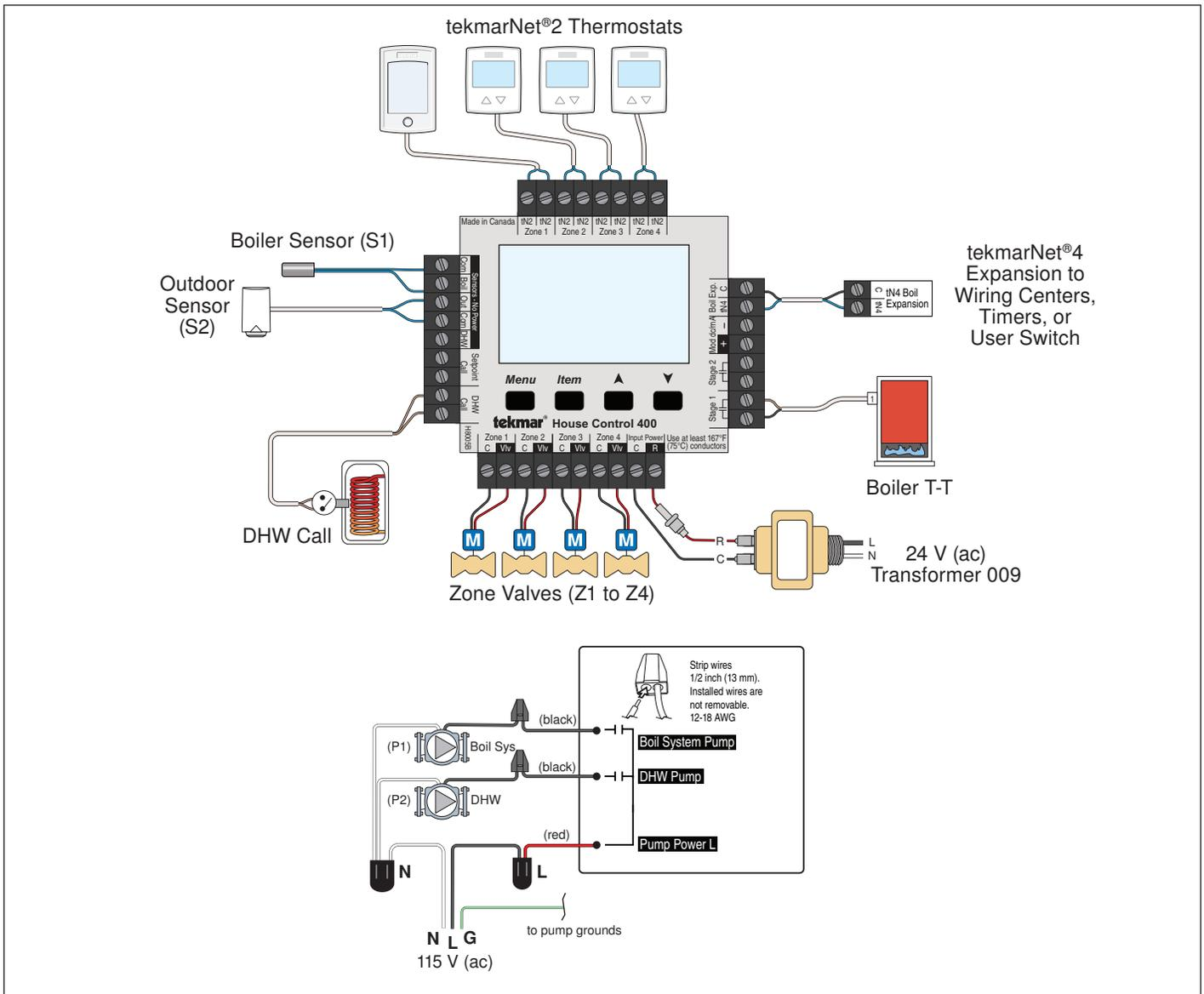
**Description:** The House Control 400 operates a modulating boiler with indirect Domestic Hot Water. The House Control 400 operates using Outdoor Reset and Indoor Feedback, which supplies the lowest water temperature to eight hydronic zones. The four extra zones are connected to the Wiring Center 313 using the tN4 Boiler Expansion terminals.
