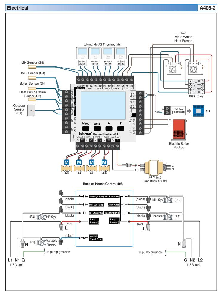
**Description:** The House Control 406 operates a water source heat pump in heating or cooling mode to supply an outdoor reset water temperature to 4 on board tank temperature zones. The 406 also operates a modulating condensing boiler to supply an outdoor reset water temperature to 4 boiler zones connected to the Boil expansion terminals with a Wiring Center 313. The boiler supplies backup heat to the tank loop using the transfer pump P7.
