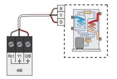
• B = Heat pump normally operates in cool mode. Energize B to operate the heat pump in heat mode
