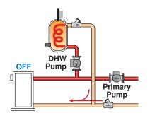
If DHW heating is to be incorporated into a low temperature system such as a radiant floor heating system, a mixing device is often installed to isolate the high DHW supply temperature from the lower system temperature. If a mixing device is not installed, high temperature water could be supplied to the low temperature system while trying to satisfy the DHW demand. This may result in damage to the low temperature heating system.
