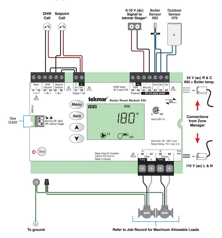
Wiring the Control Terminals 51-69
