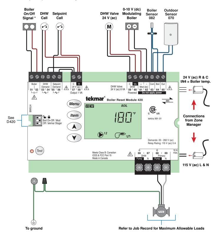
**Description:** Outdoor Reset, DHW Pump, Setpoint, Multi-stage Boiler Control.
