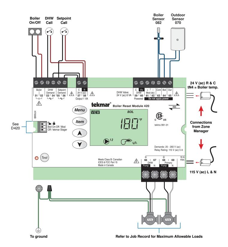
Description: Outdoor Reset, DHW Valve, Setpoint, Single 0-10 V (dc) Modulating Boiler.
