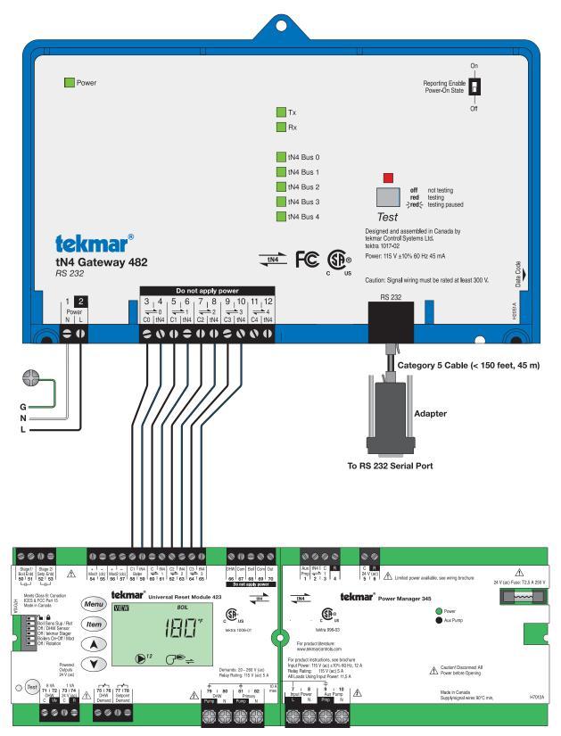
Refer to W423 and W345 wiring brochures for complete wiring schematics.
