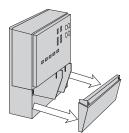
The wiring cover pulls straight out from the wiring chamber.
