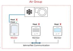
When the air group master is in cooling operation, the air group member thermostats do not operate the heating system for air heating. Once the cooling system shuts off, heating is available if required.
