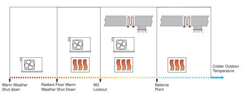
The first stage operates on a temperature differential of  $\pm 0.7$ °F ( $\pm 0.4$ °C) centered around the heating setpoint. The second stage heat turns on when the temperature drops 0.7°F - W2 Differential setting below the heating setpoint. The second stage is shut off once the temperature reaches the heating setpoint.
