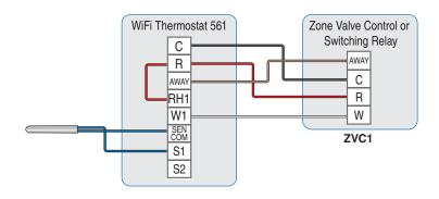
The WiFi Thermostat 561 operates a radiant floor heating system. The thermostat uses both air and floor temperature sensors. The air temperature sensor can be either built-in and/or external.
