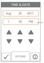
The time and date can be manually set by highlighting a field and then using the  $\blacktriangle$  or  $\checkmark$  buttons.
