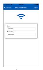
Step 5 Enter the 8 digit code from the thermostat into the mobile app. Then enter the thermostat's room name.
