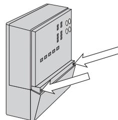
Loosen the screws at the front of the wiring cover.
