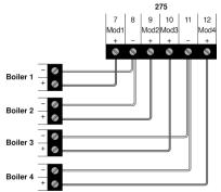
3. In the Adjust menu, select the correct Boiler Mode setting.
