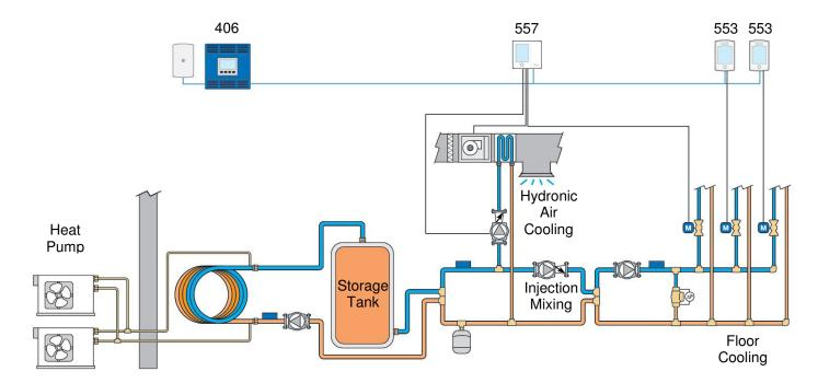
A hydronic heat pump provides both heating and cooling to a system. A storage tank acts as a buffer and reduces short cycling on the heat pump compressor. There are three floor heating and cooling zones. There is also a hydronic chilled water fan coil unit that provides air cooling and dehumidification for the entire building.
