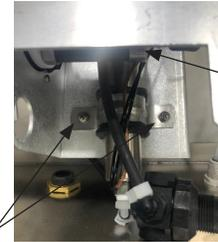
8. Remove plastic hose clamps from 90° elbows, then remove tubing from the elbows.
