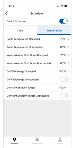
The Schedule allows you to save energy by lowering the temperature or ignoring domestic hot water calls during unoccupied time periods.
