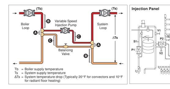
This panel shows a typical piping arrangement for a variable speed injection pump system.
