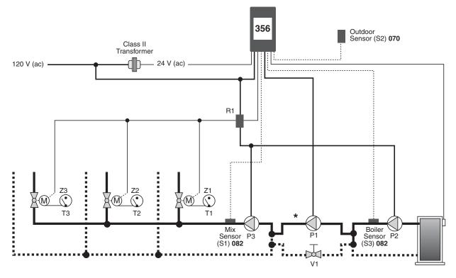
\*Read the 'Piping for Variable Speed Injection Mixing' section in the Sequence of Operation for important details about pipe diameters and spacing.
