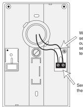
Wires from outdoor sensor to control's outdoor sensor and sensor common terminals
