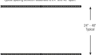
Each row of QuadRail™ must remain perpendicular to the tubing to prevent tubing from binding.
