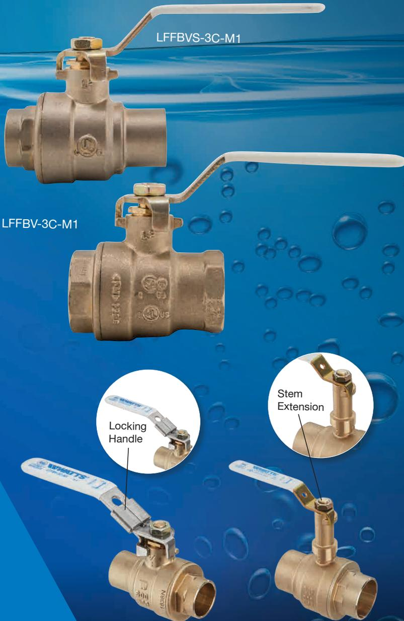
Boasting a bottom-loaded blowout proof stem, virgin PTFE seats, thrust washer, and adjustable stem packing gland, the Series LFFBV-3C-M1 2-piece, full port, Lead Free\* ball valves comply with Lead Free\* construction and can be used in commercial and industrial applications.
