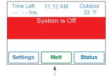
Press Melt button to start melting operation
