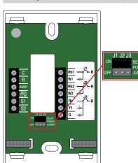
The thermostat includes three relay power jumper connectors located below the wiring hole.
