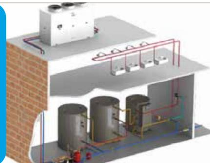
The Aegis® Heat Pump is a highly efficient heat pump water heater that uses electricity and natural CO2 refrigerant to produce domestic hot water. Its CO2 refrigerant, R744, is non-toxic, non-flammable, has an ODP (Ozone Depletion Potential) of zero and a low GWP (Global Warming Potential). Aegis® saves an estimated 144 tons of CO2 annually.
