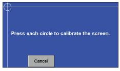
The screen has been factory adjusted but can be adjusted if the alignment is off. The screen may need to be calibrated if new software has been downloaded. It is a 5 position setup.
