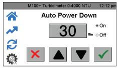
The M100+ can be set to power down automatically. The factory setting is to power down after 30 minutes. This setting is recommended to save lamp life. There is also an option to manually power off the instrument.
