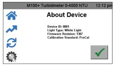
This menu shows the current setting of the Device ID, the lamp type and firmware revision number. Firmware revision can be compared to available firmware revisions on the website.
