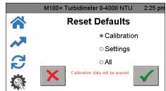
This menu allows resetting the calibration and/or settings. This clears the calibration and new calibration will be required to operate the instrument. Settings may also change, so these should be checked as well.
