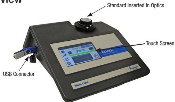
The M100+ is a process turbidimeter that allows for the laboratory measurement of the turbidity of sample water. The white light M100+ has been designed to meet the design criteria specified by the US EPA 180.1 on turbidity measurement. The infrared M100+ was designed to meet the criteria specified in ISO 7027 and DIN 27027 for the measurement of the turbidity of a sample. Both models have long life lamps.
