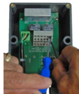
Figure 6: Electrical Connections on Terminal Block (P1)
